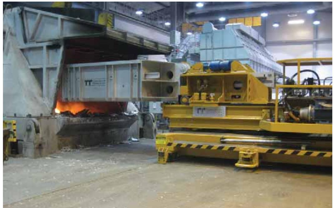
Figure 3. With the furnace door open the charging box is automatically rammed into the furnace to discharge the scrap for melting. After discharge of the scrap the system will return to the loading bay to await the loading of more scrap.
