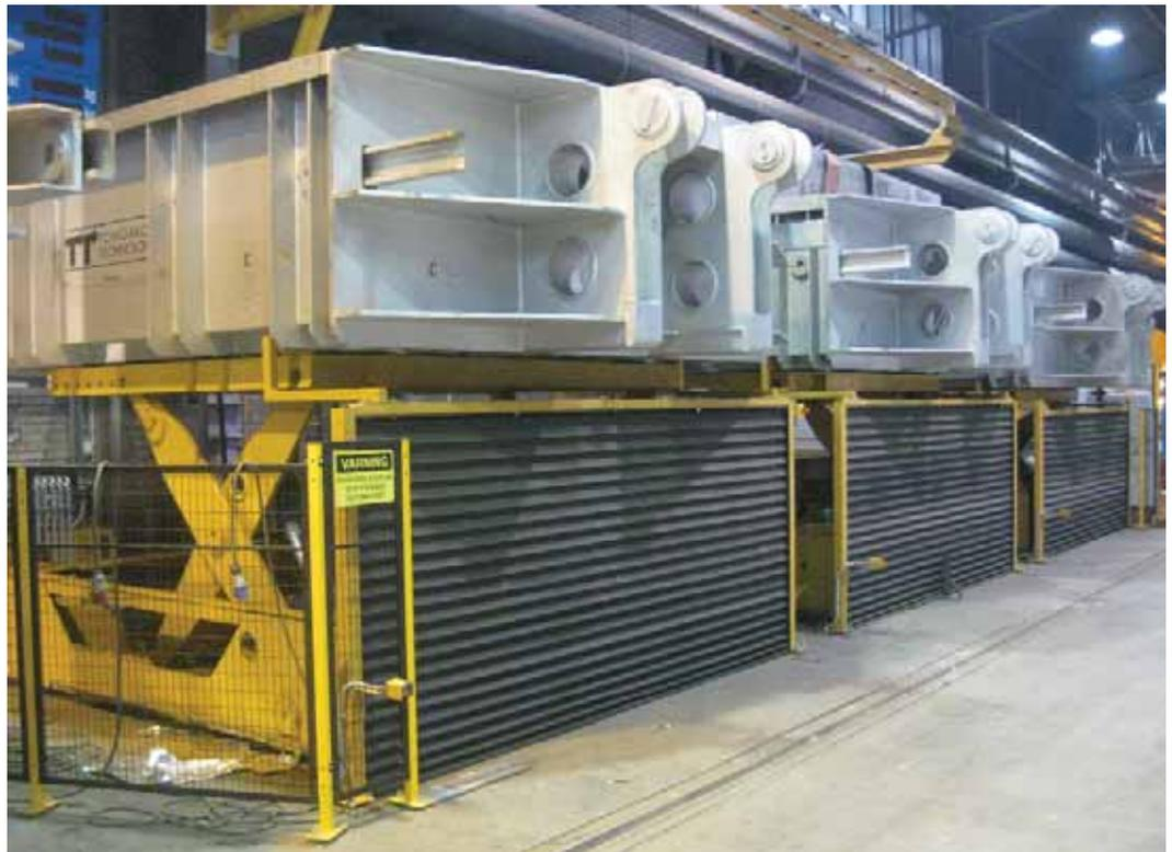
Figure 2. After scrap loading the charging boxes travel to the unloading position in front of the furnaces and automatically discharge their load into the furnace.
