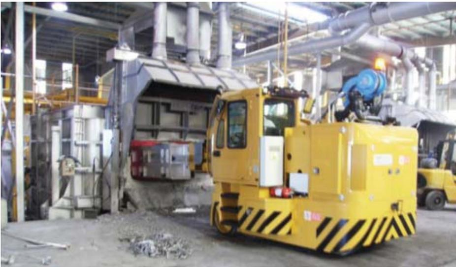
4 T.T. Tomorrow Technology Furnace Charging Vehicles have their own weighing system on board each vehicle.
