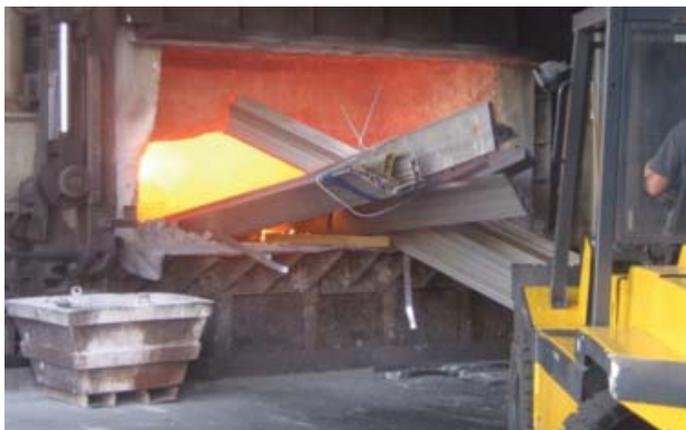
2 Thesetwo pictures are typical of the method used in many cast houses to load the aluminium melting furnaces.
