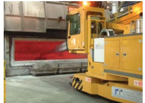
6 Furnace tending vehicles built by T.T Tomorrow Technology (this picture shows a telescope length reach of 9.5 metres) are much more efficient than the standard forklift and dumpers truck for skimming and cleaning operations.
