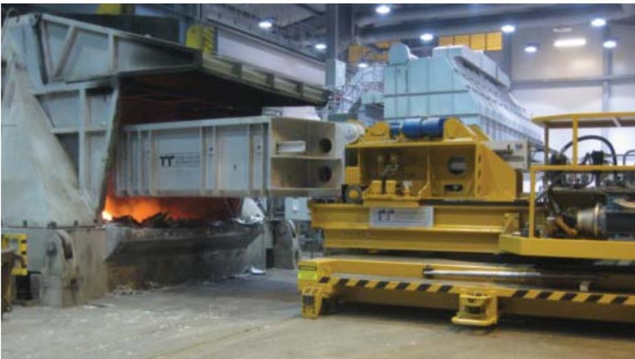
5 A fully automated scrap management system and furnace charging machine of 10 tons capacity at Sapa Finspang (Sweden). The picture shows the furnace door open and the charging box is automatically rammed into the furnace to discharge the aluminium scrap for melting. After discharge of the scrap the system will return to the loading bay to await the loading of more scrap. Notice the rails for the furnace charging machine to travel on, can be seen on the works floor.
