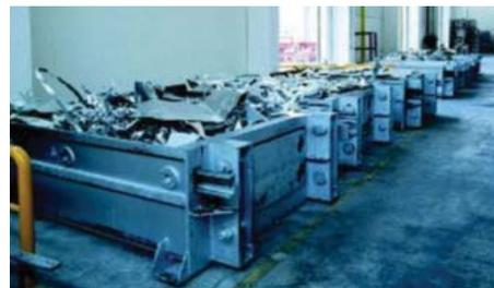
3 Charging boxes loaded with scrap ready for furnace.
