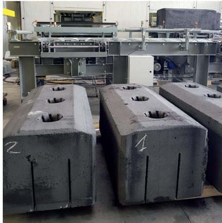
bubbles ( $\text{CO}_2$ ,  $\text{CO}$ ) released at the bottom of the anode during the electrolysis process, thereby reducing production costs and improving metal output. Especially for the Norwegian project, the standard core of T.T.'s design was adapted to the specific Alcoa requirements in order to be smoothly integrated in the Norwegian anodes production facility. The ability to cut slots with interrupted profiles (to direct released gas to the centre of the pots)
