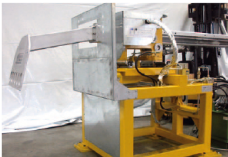
Fixed furnace cleaning, metal mixing and bottom clearing equipment
