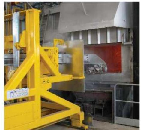
T. T. Tomorrow Technology rail-mounted de-drossing equipment operating at the hot chamber of a twin-chamber melting furnace.
