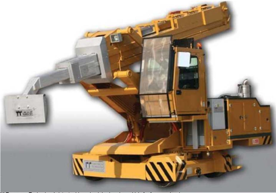
TT Tomorrow Technology's latest rubber wheel de-drossing vehicle for furnace cleaning
