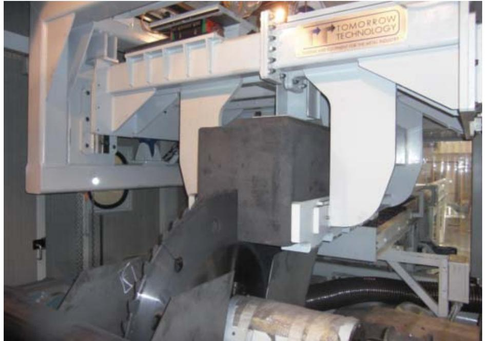
2 Single slot cut by automatic anodes slotting line
