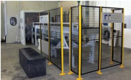
1 Automatic anodes slotting line manufactured by the Italian company T. T. Tomorrow Technology.
