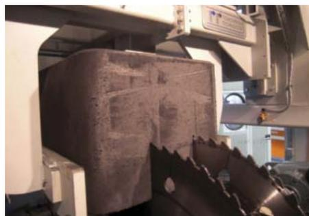
3 Twin slots are cut in a big anode by the automatic anodes slotting line
