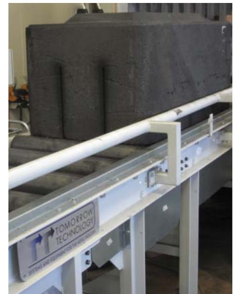
4 The discharge conveyor with anodes after 2 deep slots having been cut
