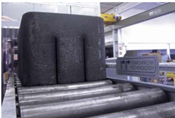
The second method – cutting slots into the anodes after the baking process – overcomes the limits and disadvantages of slots formed during vibro-compaction.
