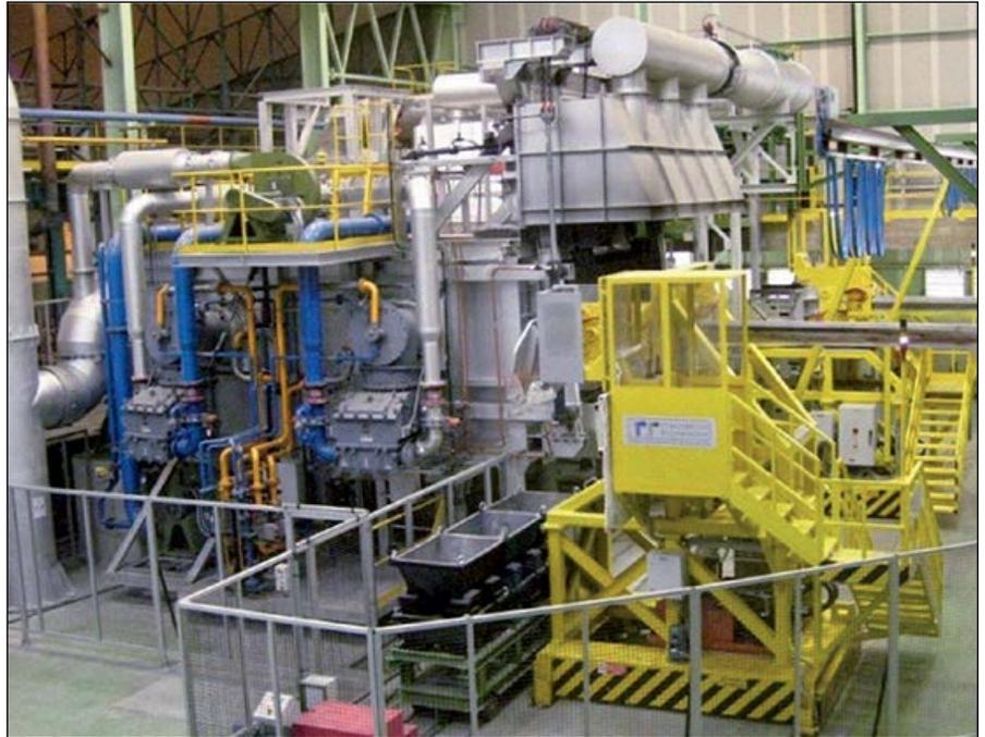
Figure 1. A new generation of automatic tending systems on rails are able to perform multiple functions, including charging, skimming, alloying, and furnace cleaning.
