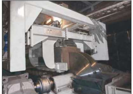
Figure 2. Anode slotting machine.
